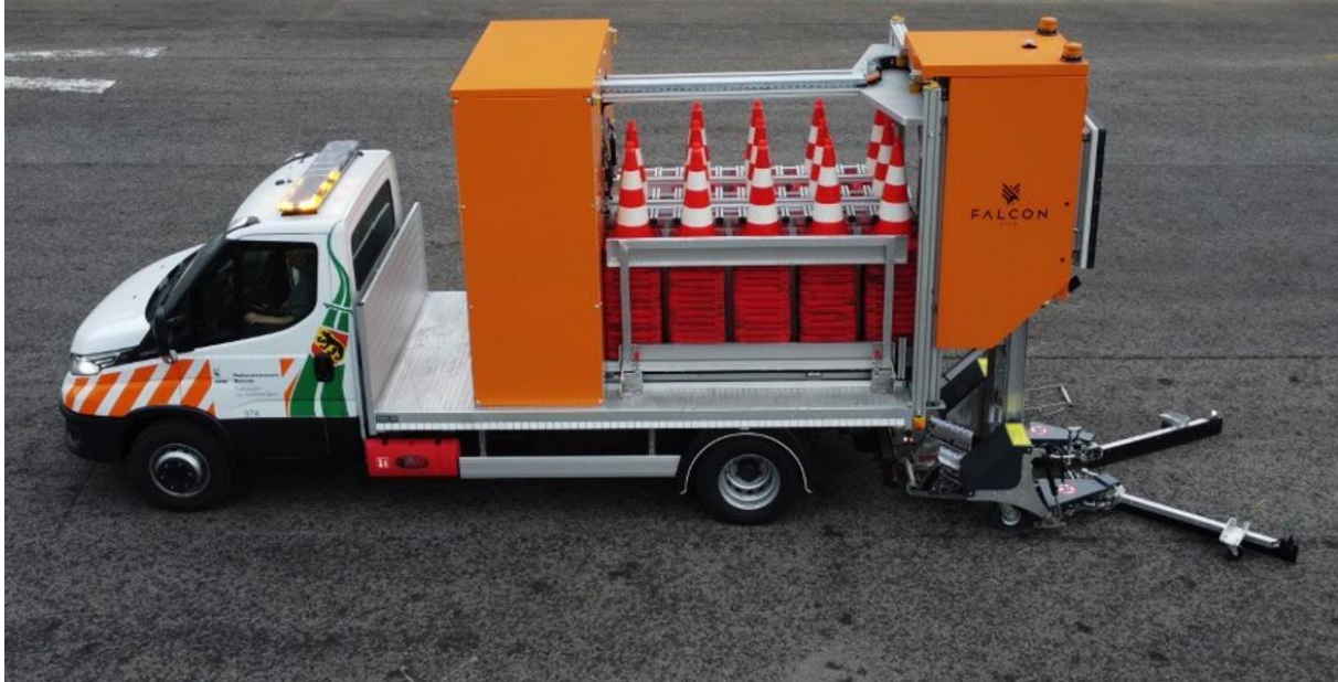
Figure 1: Falcon 75 on an Iveco Daily 70 chassis
